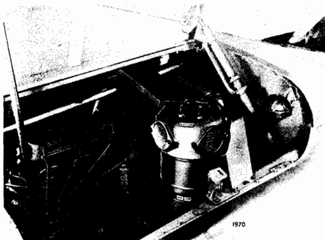
Under-bonnet Installation of Universal Oil Bath Type Air Filter on a Double-Deck Passenger Vehicle
